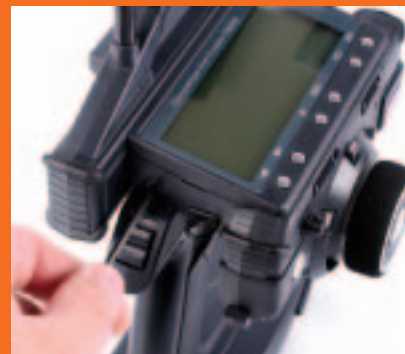
Reinstall the 4mm hex screws to finish the job. Just snug them up; don't overtighten.
