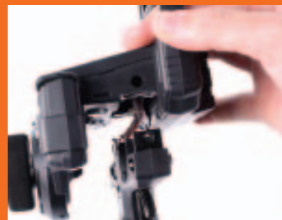
Separate the transmitter body from the grip body by simply pulling them apart.
