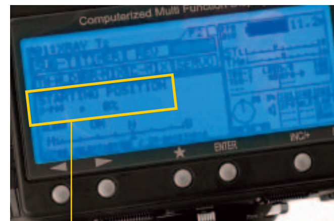
Set the Starting Position by inputting a percentage of full throttle. For example, 10% would hold the engine at 1/10 of full throttle.
