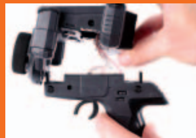
Rotate the transmitter body 180 degrees, and lower the transmitter body back down onto the grip body. Be careful not to damage the wires by pulling them out too far or by pinching them between the transmitter body and grip body.
