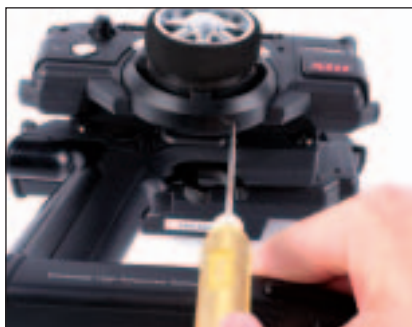
Trigger and wheel tension settings let you customize the M11's feel.
