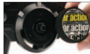
Keep the dirt out by covering the wheel bearing.
