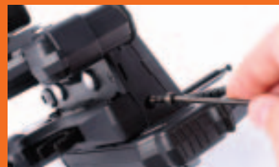
Remove the two 4mm hex-head screws with a 3mm hex-wrench, one on each side of the radio.
